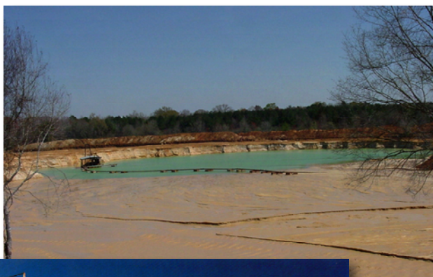
Open pit dredging activities - MMM wash plant return into an active dredge pit
