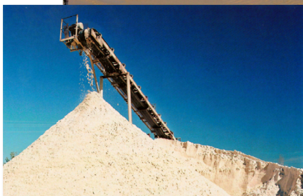
Wet/Dry processing – MMM conveyor depositing sand separated through the processing plant
