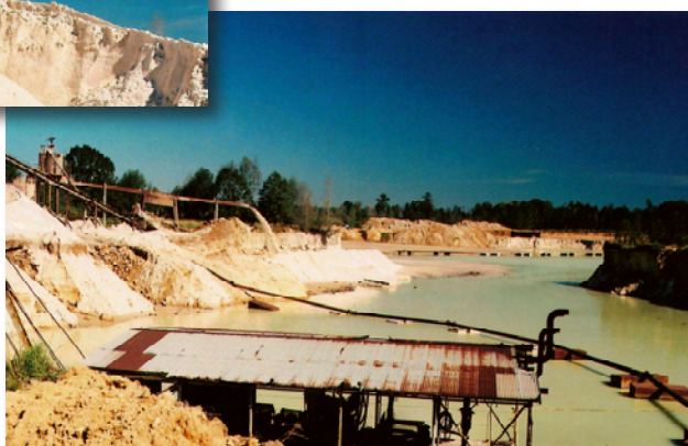
Dredging activities - MMM photo of dredge in active dredge pond (forefront) with Wash Plant in background
